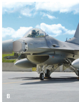
(A) B-2 Radar Modernization Program antenna undergoing test and verification at the Raytheon systems integration lab. (B) Raytheon Advanced Combat Radar (RACR) brings scalable AESA capability to multiple fighter aircraft. (C) The Multi-Function Radio Frequency System, shown in production, provides crucial radar and fire control input for Raytheon's Active Protection System.
