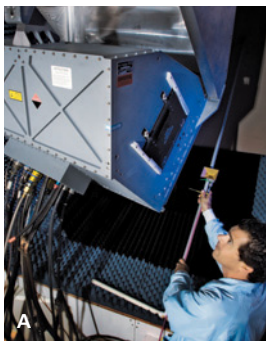
(A) B-2 Radar Modernization Program antenna undergoing test and verification at the Raytheon systems integration lab. (B) Raytheon Advanced Combat Radar (RACR) brings scalable AESA capability to multiple fighter aircraft. (C) The Multi-Function Radio Frequency System, shown in production, provides crucial radar and fire control input for Raytheon's Active Protection System.
