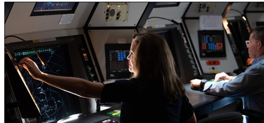
Air Traffic Controllers in Terminal Radar Approach Control stations use STARS to provide safe and efficient aircraft spacing and sequencing guidance for departing and arriving aircraft in airports and U.S. military terminal areas. Raytheon Intelligence & Space is partnering with both the Federal Aviation Administration and the Department of Defense to implement the terminal automation systems in airports as part of the FAA's NextGen modernization plan for the National Airspace System.
