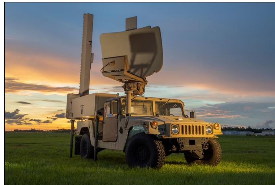
The U.S. Air Force awarded the Lightweight Deployable-Ground Controlled Approach contract on March 11. LD-GCA provides the Air Force with an upgrade to our Air Traffic Navigation, Integration, and Coordination Systems, or ATNAVICS. The LD-GCA system ensures autonomy and extends the Primary Surveillance Radar range to 60-nautical-miles without increasing the system footprint.
